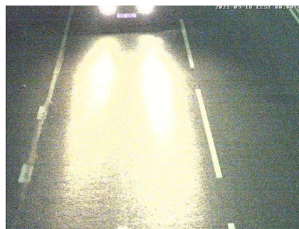
Fig. 6. Example of an image that cannot be used for number plate recognition
